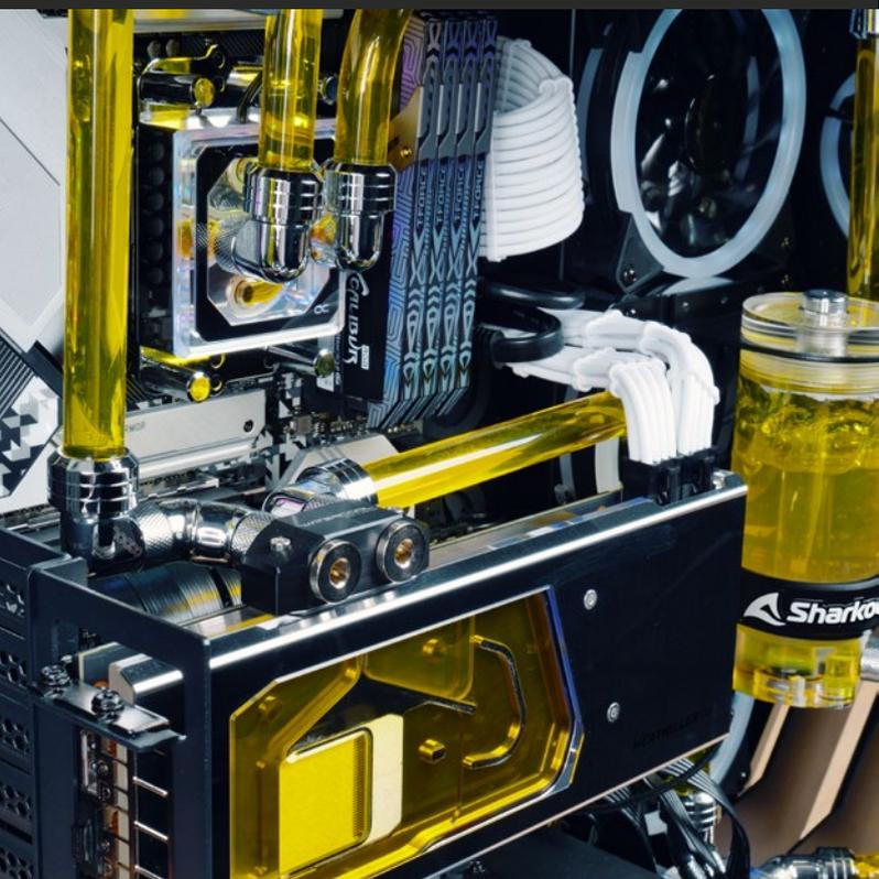
Of course, the interior of the ELITE SHARK CA700 can also be water cooled. However, what is special about the case is the possibility of installing two 360 mm radiators at the same: one in the top of the case and another next to the mainboard.
