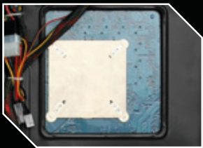
Mainboard backplate with installation opening for CPU coolers
