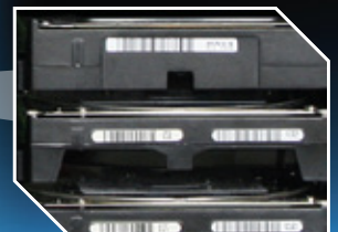
5x 3,5" bays for HDDs and screw-mounted cage
