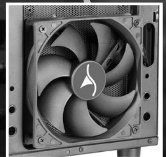
120 mm front fan with dust filter
